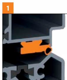
THE ADDITIONAL EPDM GASKET SEALS THE CONNECTION BETWEEN THE LEAF AND THE THRESHOLD
