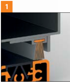
1 ADDITIONAL BRUSH SEAL SEALING THE JOINT OF THE LEAF AND THE THRESHOLD
