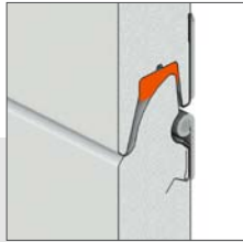
Panel with a thickness of 40 mm. U=1,12 \text{ [W/m}^2\text{K]}^*
