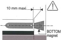
Operate the door to a mid position and then connect the ESE safety edge connector to the ESE safety edge transmitter terminal as illustrated.
