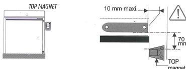
Operate the door to the closed position and secure the BOTTOM ESE transmitter magnet to the guide rail:
